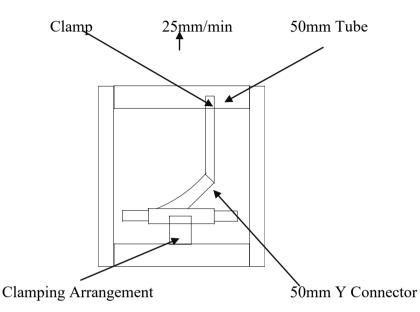
Prepare an assembly as above and using a suitable clamping arrangement secure the 50mm protective tube section to one of the tensometer jaws. Place the branch tube in the other jaw and perform a destructive test at a rate of extension of 25mm/minute.
